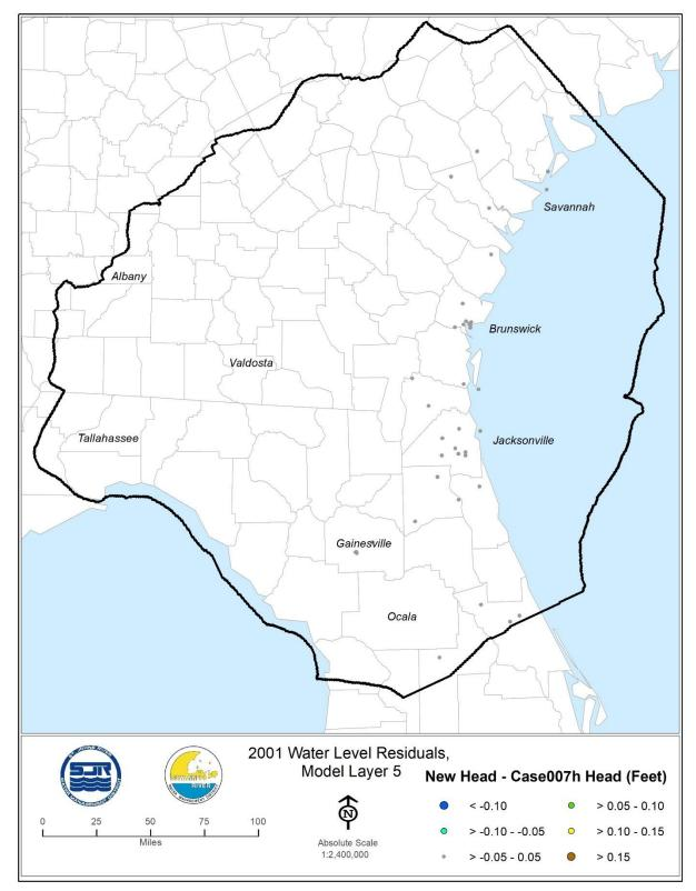
Figure 22. Head difference (in feet) at Model Layer 5 observation targets, 2009. The head difference was calculated by subtracting the case007h simulated head from the case007h-1 simulated head.
