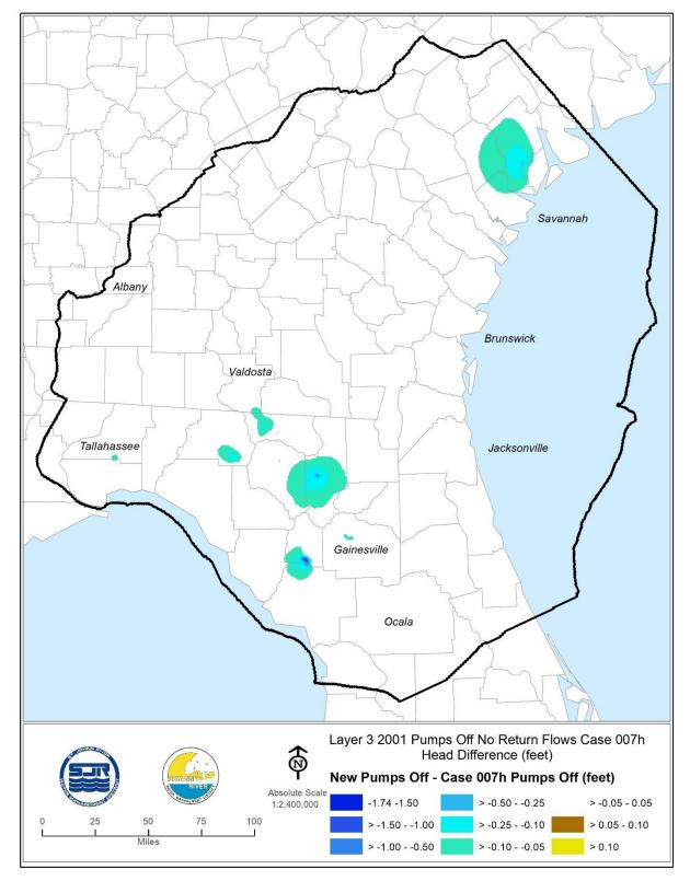
Figure 33. No-pumping head difference (in feet) in Model Layer 3, 2001. The head difference was calculated by subtracting the case007h simulated head from the case007h-1 simulated head.
