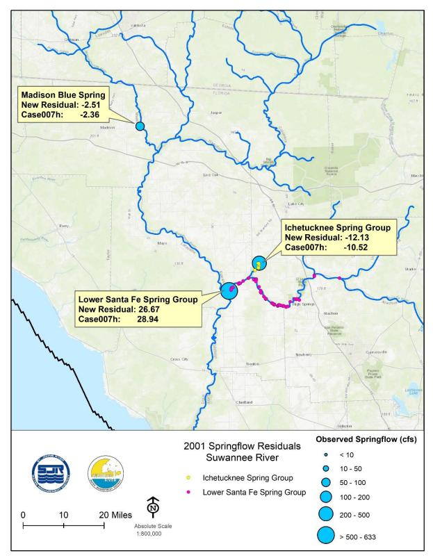
Figure 8. Comparison of residual spring flow at selected springs, 2009. The residual was calculated by subtracting the estimated spring flow from the modelled spring flow.
