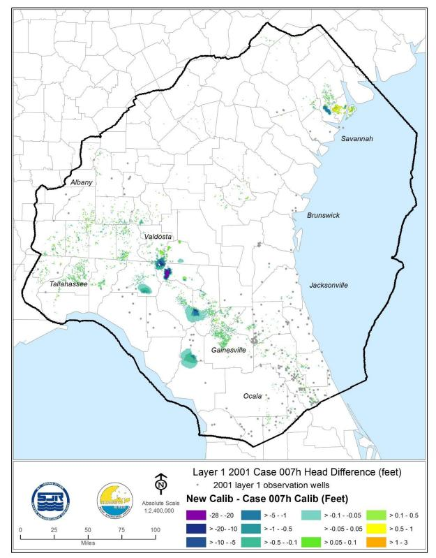
Figure 11. Head difference (in feet) at Model Layer 1 observation targets, 2009. The head difference was calculated by subtracting the case007h simulated head from the case007h-1 simulated head.
