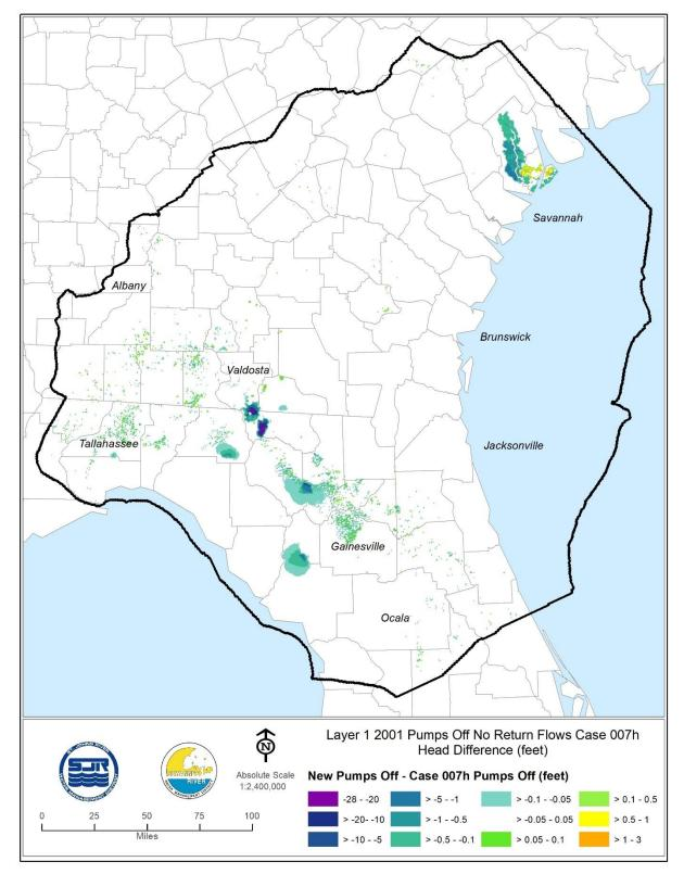
Figure 31. No-pumping head difference (in feet) in Model Layer 1, 2001. The head difference was calculated by subtracting the case007h simulated head from the case007h-1 simulated head.
