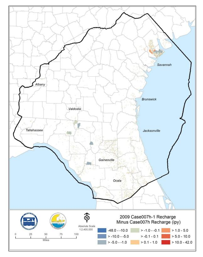
Figure 2. Difference in recharge in inches per year, 2009. The difference in recharge was calculated by subtracting the case007h recharge from the case007h-1 recharge.
