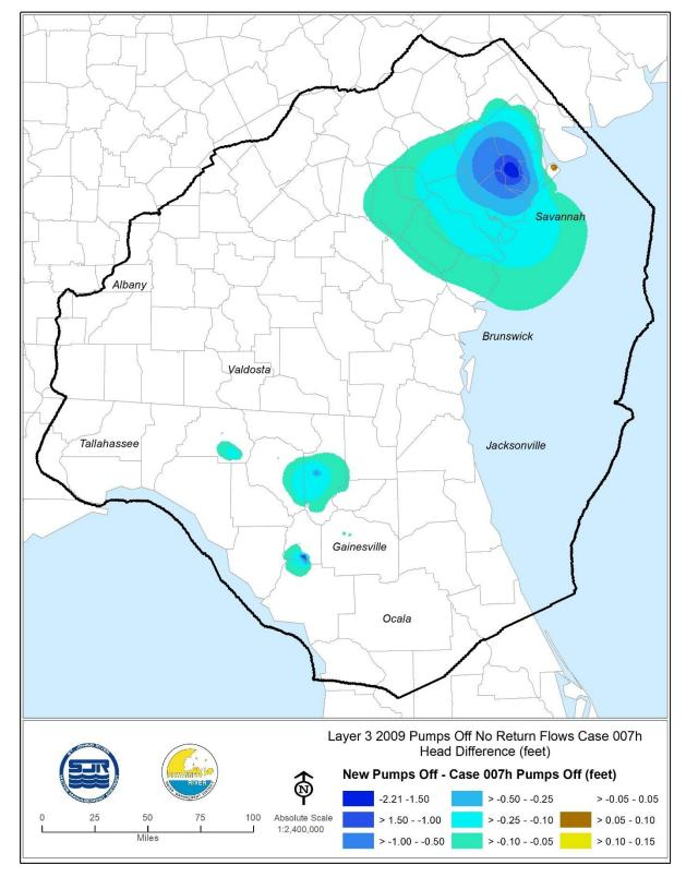
Figure 34. No-pumping head difference (in feet) in Model Layer 3, 2009. The head difference was calculated by subtracting the case007h simulated head from the case007h-1 simulated head.
