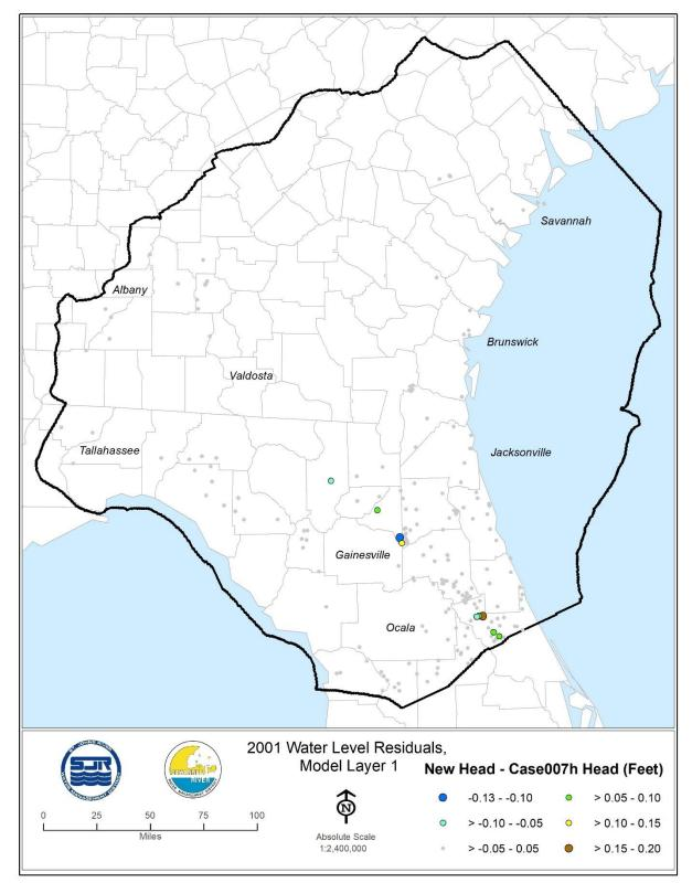
Figure 10. Head difference (in feet) in Model Layer 1, 2001. The head difference was calculated by subtracting the case007h simulated head from the case007h-1 simulated head.
