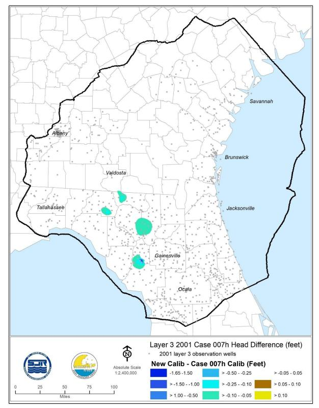
Figure 17. Head difference (in feet) at Model Layer 3 observation targets, 2009. The head difference was calculated by subtracting the case007h simulated head from the case007h-1 simulated head.
