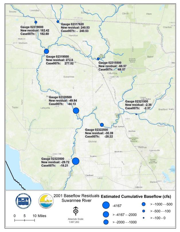
Figure 24. Comparison of cumulative baseflow rate residuals for selected USGS gauges, 2009. The residual was calculated by subtracting the estimated baseflow rate from the modelled baseflow rate.
