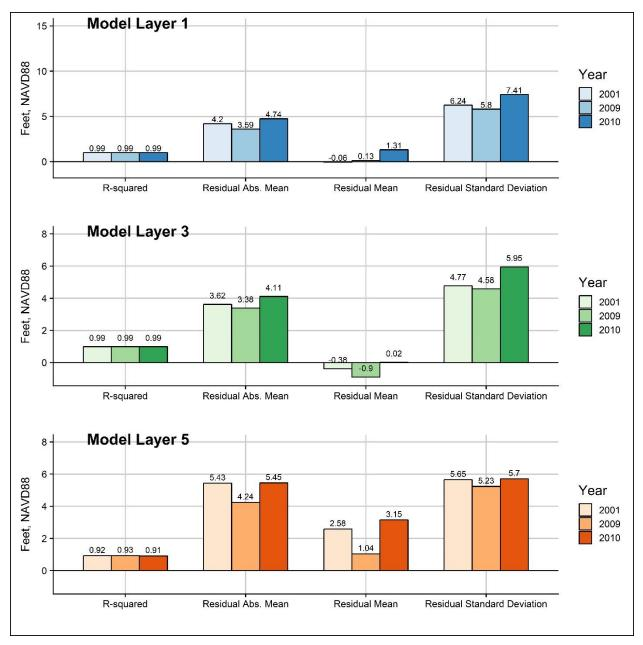
Figure 37. Comparison of case007h-1 groundwater level residual statistics at observation targets for Model Layers 1, 3 and 5 in 2001, 2009 and 2010.
