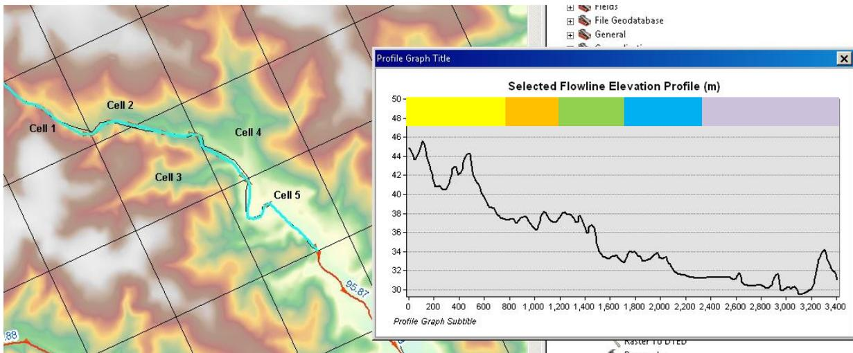
**Figure 1. Plan and Profile Example for NHD 3D Flowlines**
